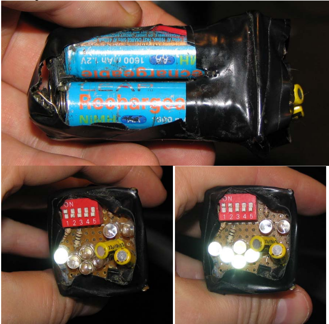
Figure 1: The first prototype. The bottom left shows the first switch switched on and the bottom right shows both the first and second switches switched on:
